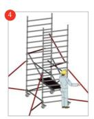
Continue diagonal bracing in a zig-zag pattern by attaching 2 diagonal braces on each side (5<sup>th</sup> to 8<sup>th</sup> and from the 8th to the 11<sup>th</sup> rungs). Fit stabilisers to the base unit - see separate section on stabilisers below.
