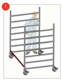
Insert castors and adjustable legs into the 7 rung frames. Clip horizontal brace onto the vertical member just above the 1<sup>st</sup> rung, with claw facing outwards.
