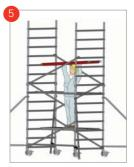
Fit trapdoor platform to the 10<sup>th</sup> rung of the tower.
